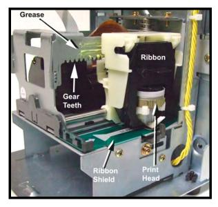
Figure 6-10. Ribbon Carriage Grease.
